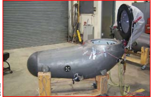
One-man submersible hull instrumented with strain gages for external pressure test to establish maximum depth capability
