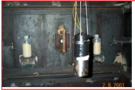
Thermobaric device to be tested in a blast chamber against simulated biological agent
