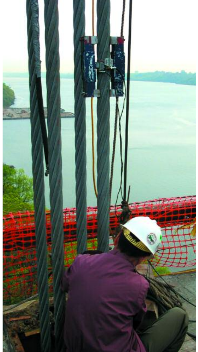
SwRI engineers built a magnetostrictive sensor system to inspect the three-inch-diameter suspenders of bridges. From one probe location, the low-cost technique detects geometric features and defects in the suspender ropes without the need for paint removal.
