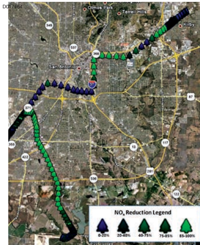
An illustration of data logger tracking during early operation of the SCR equipped locomotive in San Antonio shows placemarks shaded according to the NO x reduction recorded at each point. Areas of little or no NO x reduction are due to exhaust temperatures being below the threshold of SCR activity.
