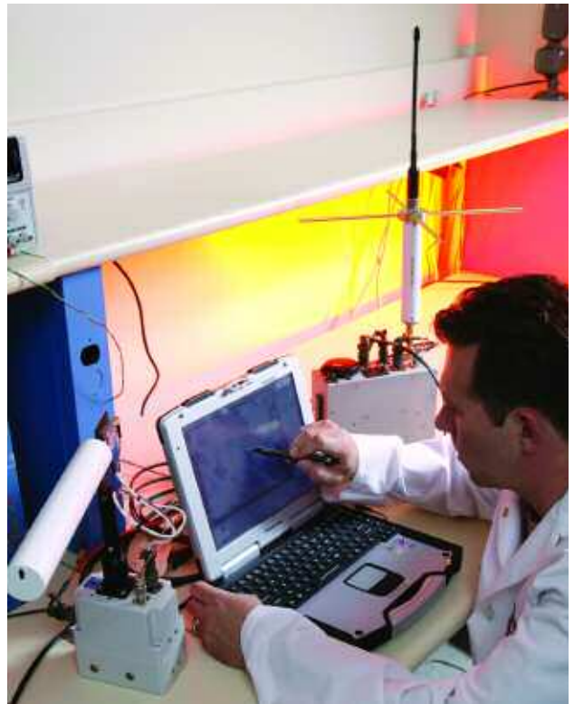
Communication and tracking antennas for Buster's ground control system, shown in the laboratory at right, can be easily mounted atop a temporary structure or a vehicle.
