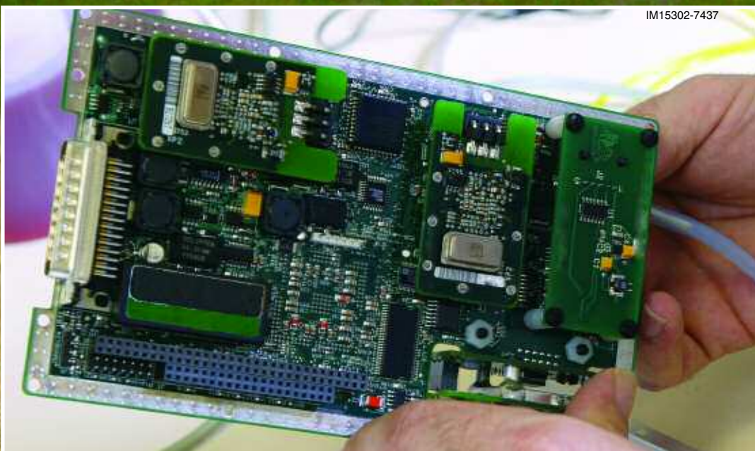
The rail-launched Buster UAS needs neither wheels nor runways, and its onboard flight management system can be held in one hand.
