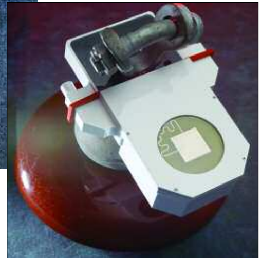
The insulator sensor is designed to fit around the Y-bolt that attaches the bell to the grounded structure. Thumb screws are used to secure the two halves of the current transformer. Leakage currents are continually monitored and peak levels are stored in a histogram.
