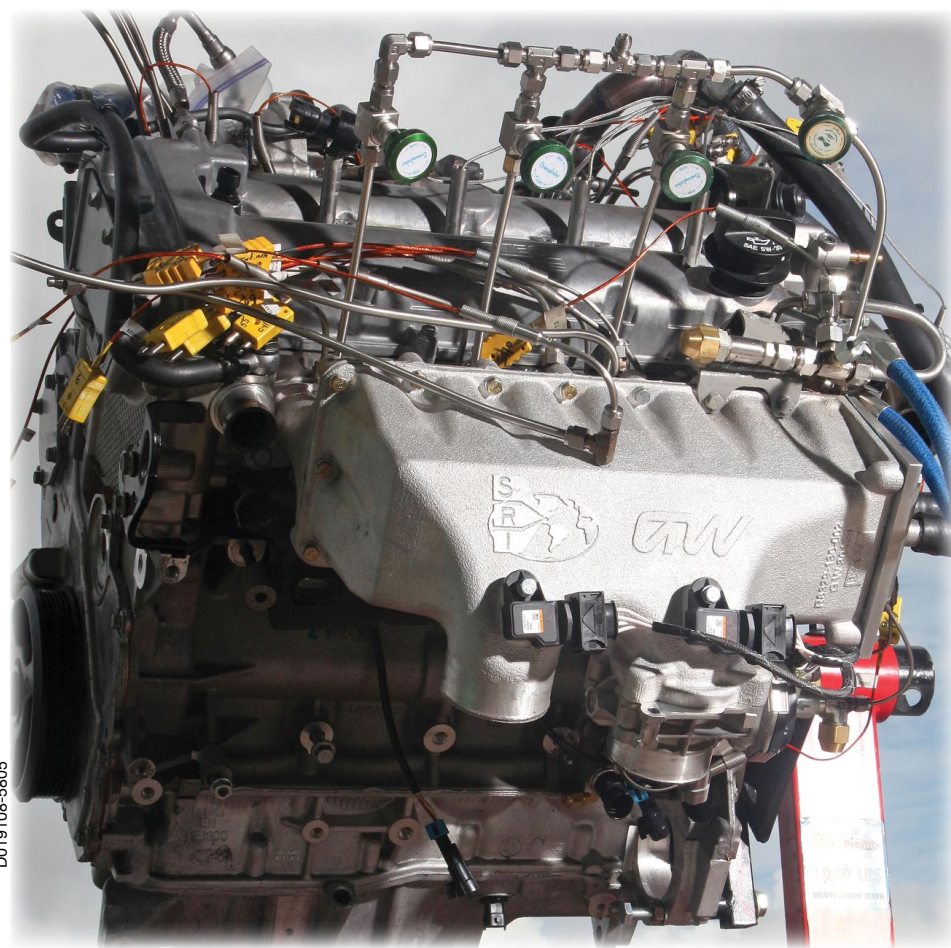
SwRI's high-efficiency D-EGR engine contains custom-designed airpath parts.
