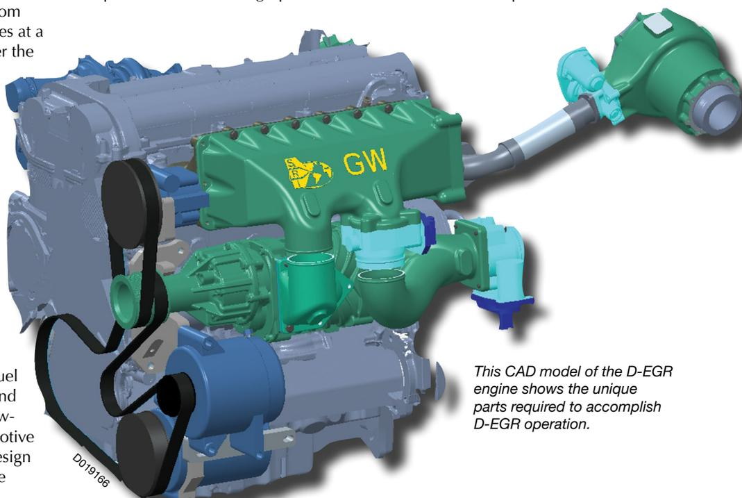
This CAD model of the D-EGR engine shows the unique parts required to accomplish D-EGR operation.
