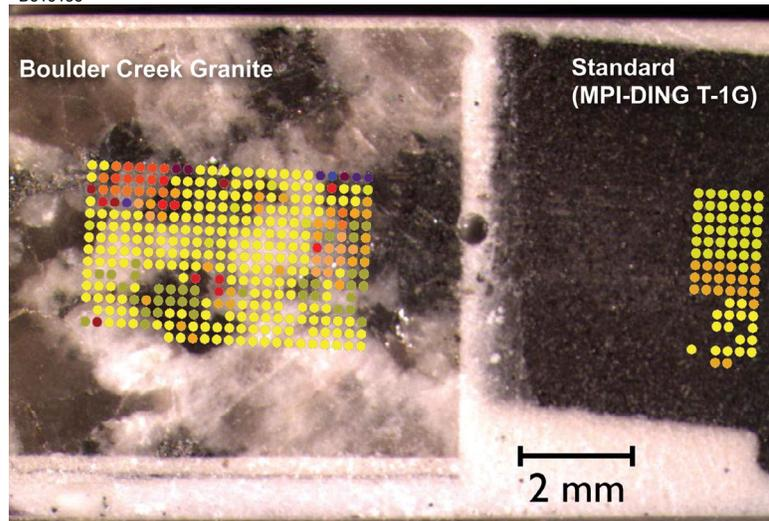
The LDRIMS-1 measured hundreds of spots on a granite sample, shown here by a group of colored dots, spaced 300 microns apart and producing microscopic pits about 75 microns wide and 0.5 micron deep.
