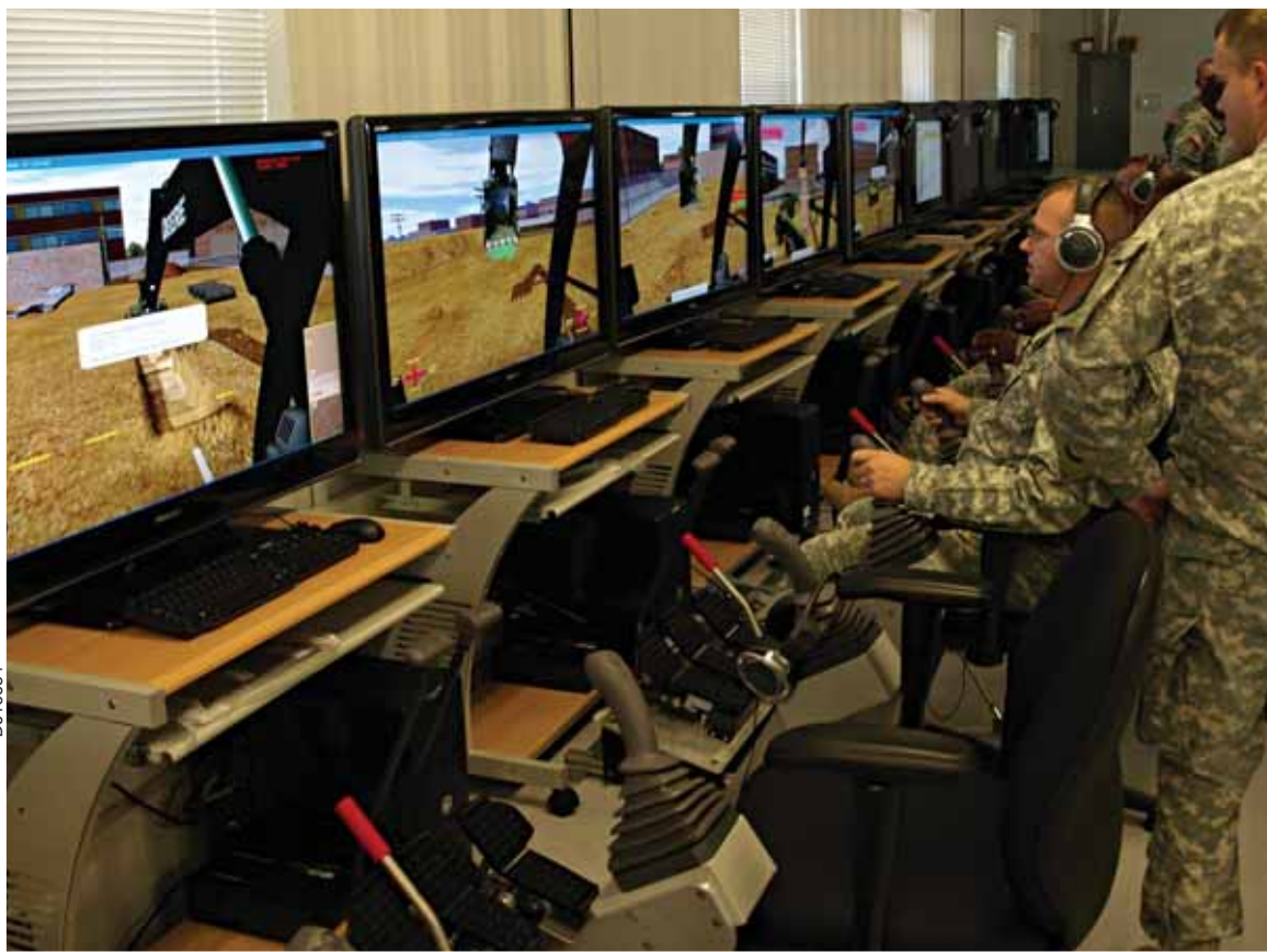
Military application of the excavator operation simulator allows trainees at multiple stations to work independently on different phases of excavation while being supervised by a single trainer.
