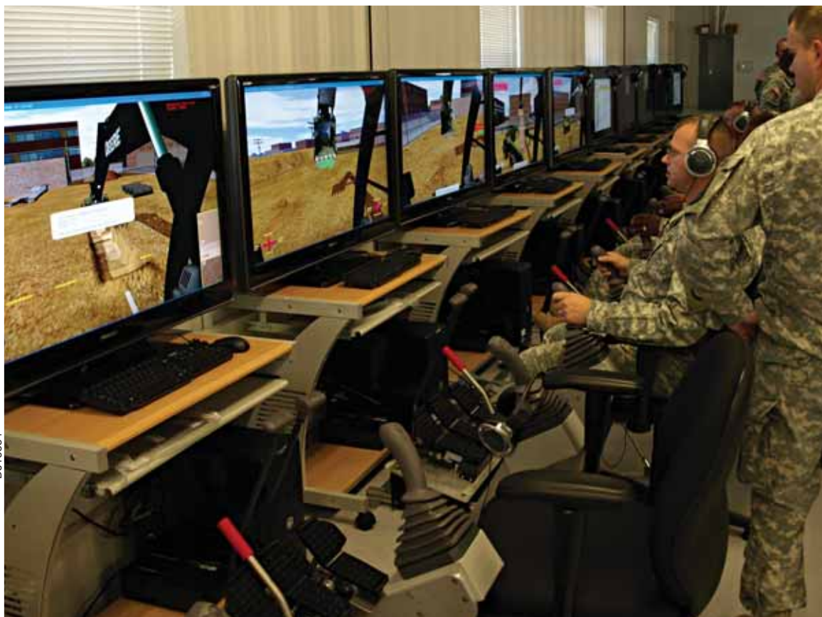
Military application of the excavator operation simulator allows trainees at multiple stations to work independently on different phases of excavation while being supervised by a single trainer.
