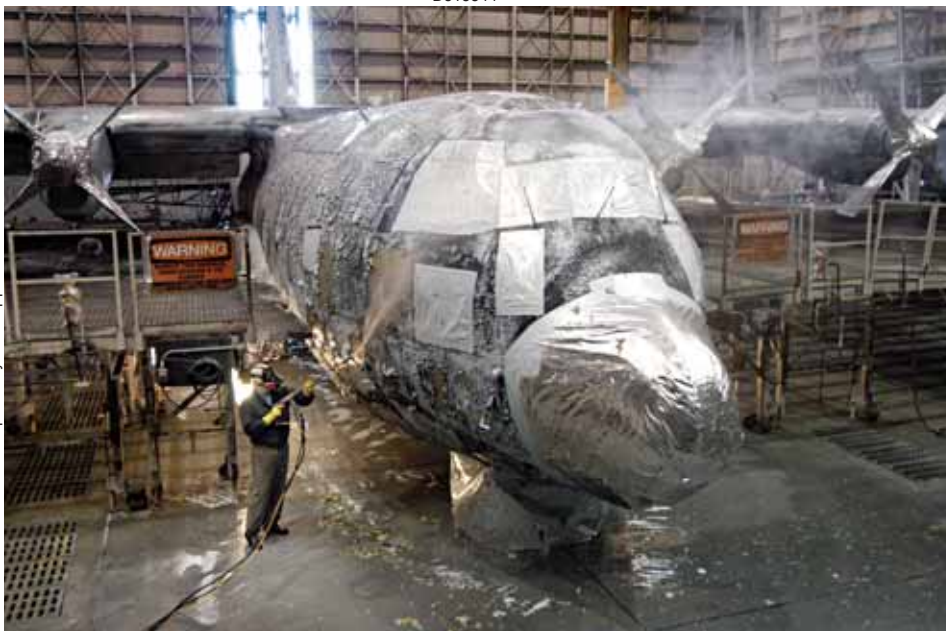
The ACRES system eliminates worker exposure to hazardous environments, such as the chemical stripping process shown above.
