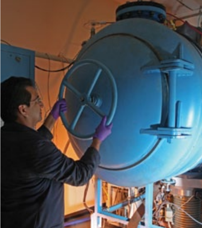
The SwRI PIID coating chamber allows multiple components to be coated simultaneously, thus lowering the cost of the coating.
