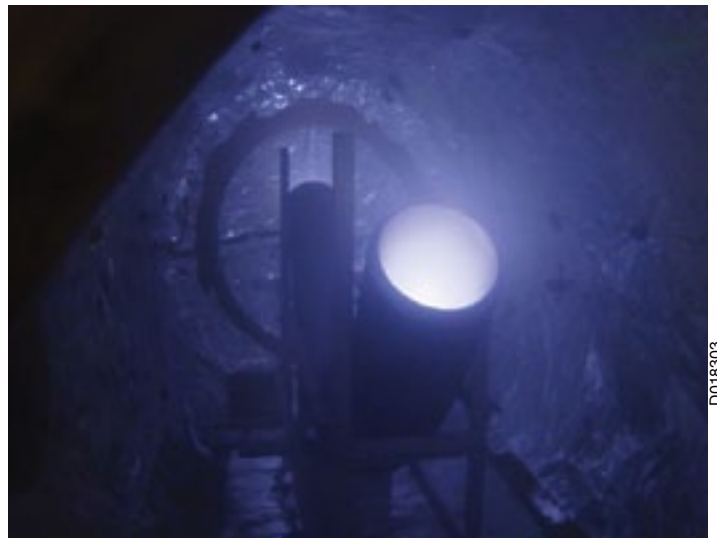
Using the hollow cathode discharge phenomenon, SwRI researchers have successfully coated curved pipes up to seven feet long and six inches in diameter.
