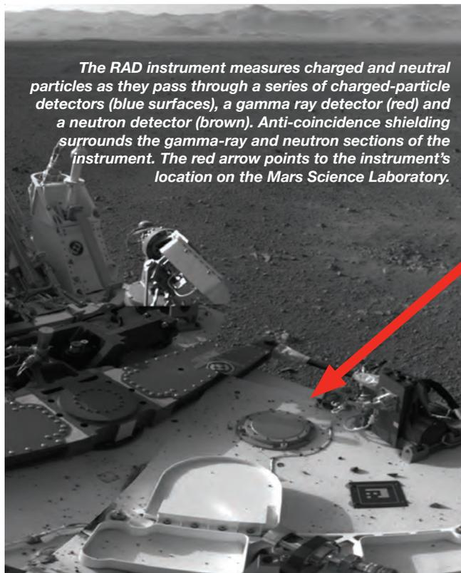
*The RAD instrument measures charged and neutral particles as they pass through a series of charged-particle detectors (blue surfaces), a gamma ray detector (red) and a neutron detector (brown). Anti-coincidence shielding surrounds the gamma-ray and neutron sections of the instrument. The red arrow points to the instrument's location on the Mars Science Laboratory.*
