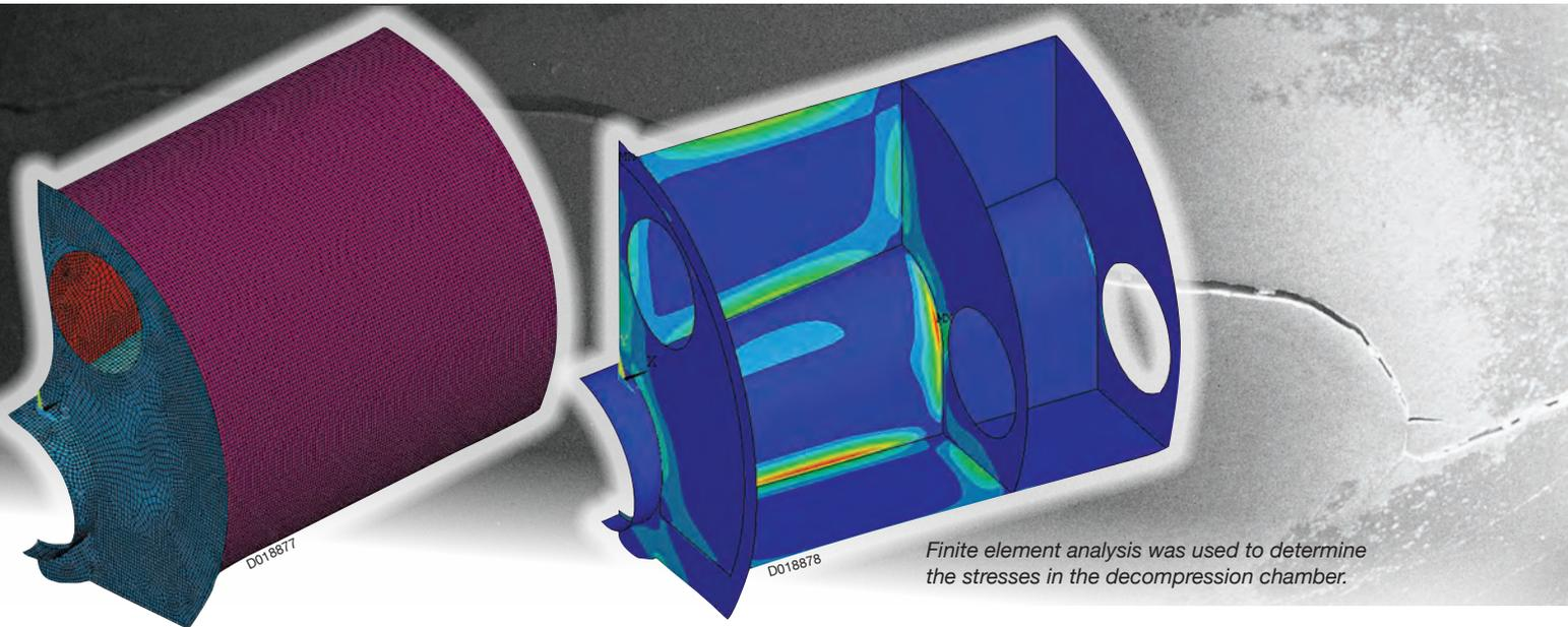
Finite element analysis was used to determine the stresses in the decompression chamber.
