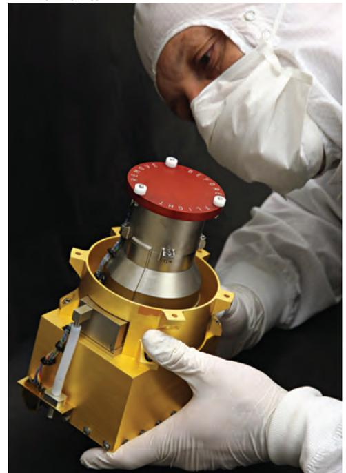
*The Radiation Assessment Detector, one of 10 instruments onboard the Mars Science Laboratory, measures fluxes of solar energetic particles and galactic cosmic rays to help assess the radiation environment on Mars, as well as on the journey from Earth to Mars.*
