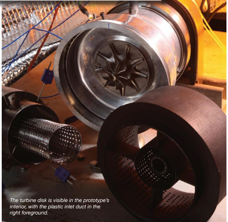
The turbine disk is visible in the prototype's interior, with the plastic inlet duct in the right foreground.
