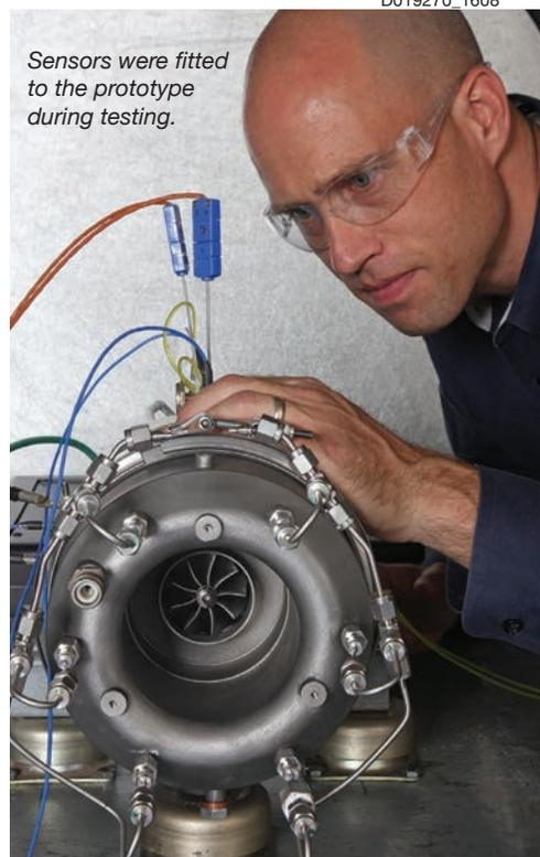
Sensors were fitted to the prototype during testing.
