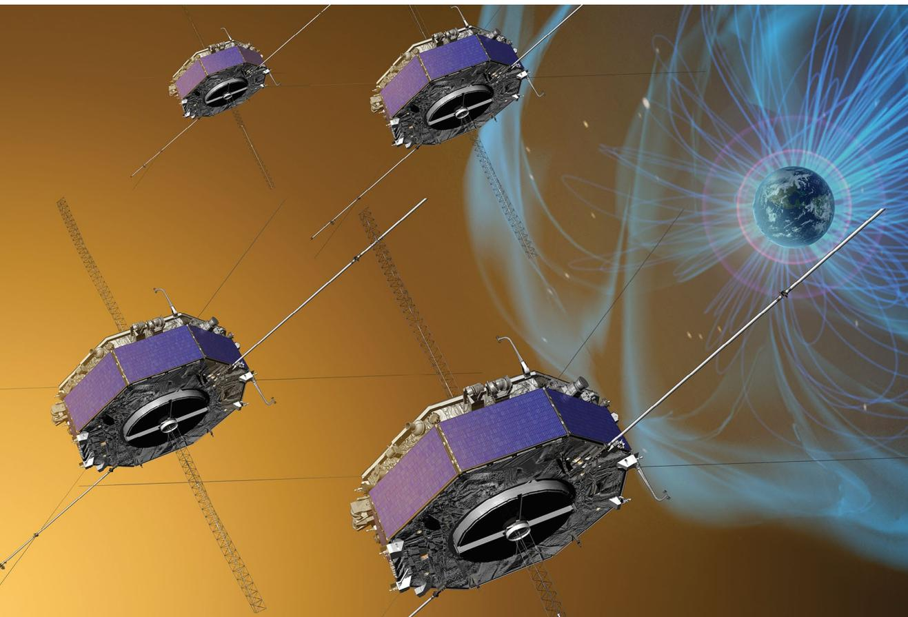
Launched March 12, 2015, the four identical MMS spacecraft skim the sunward boundary of Earth's magnetosphere in a close tetrahedral formation. Each spacecraft carries a payload of 25 instruments to measure with unprecedented resolution the plasma, energetic particles, and electric and magnetic fields near and in magnetic reconnection sites.
