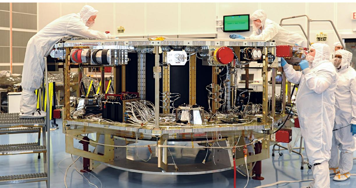
The four identical MMS spacecraft fly in formation at the boundary of the magnetosphere, collecting data at incredible rates, looking for evidence of magnetic reconnection. Here, technicians integrate the 25-instrument payload into one of the spacecraft.
