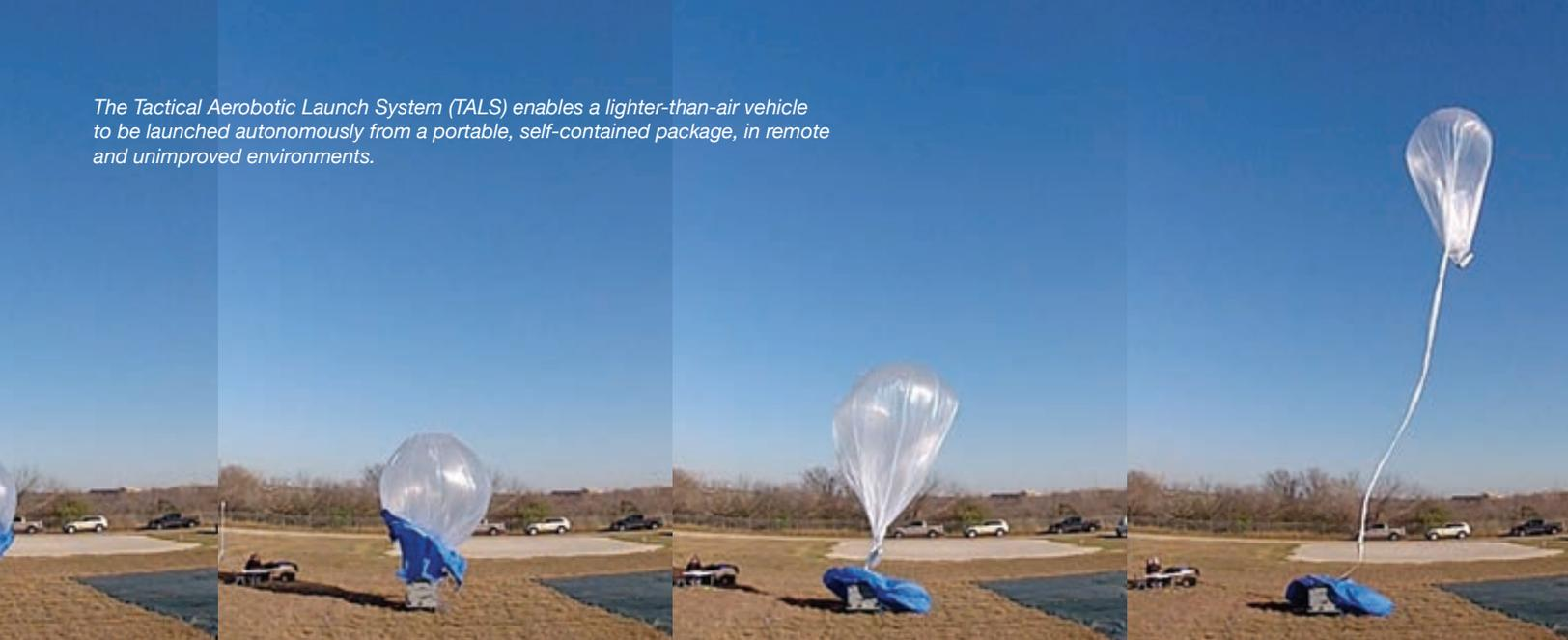
structure. Once the container is secured, the LTA system can be launched immediately or left for autonomous launch at a later time using a timer or telecommand. After launch, the container can be recovered and refurbished for reuse.
