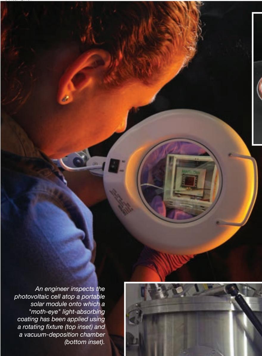
*An engineer inspects the photovoltaic cell atop a portable solar module onto which a "moth-eye" light-absorbing coating has been applied using a rotating fixture (top inset) and a vacuum-deposition chamber (bottom inset).*
