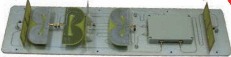
The sub-arrays—with one facing front, rear and two broadside—work together to provide 360-degree coverage. Two different antenna element types are used: balanced-shielded loop antenna elements to cover VHF frequencies and tapered-slot antenna (TSA) elements for UHF. Each sub-array design was 30 inches long by 7.5 inches tall by 3.5 inches deep for this platform.
