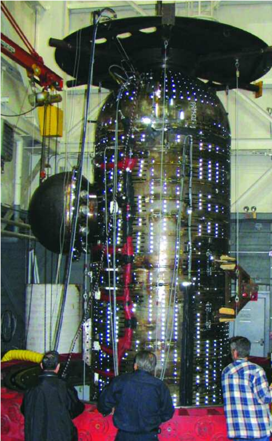
Technicians lower the rescue module hull into a deep ocean simulator at the U.S. Navy Deep Submergence Laboratory in Caderock, Md.
