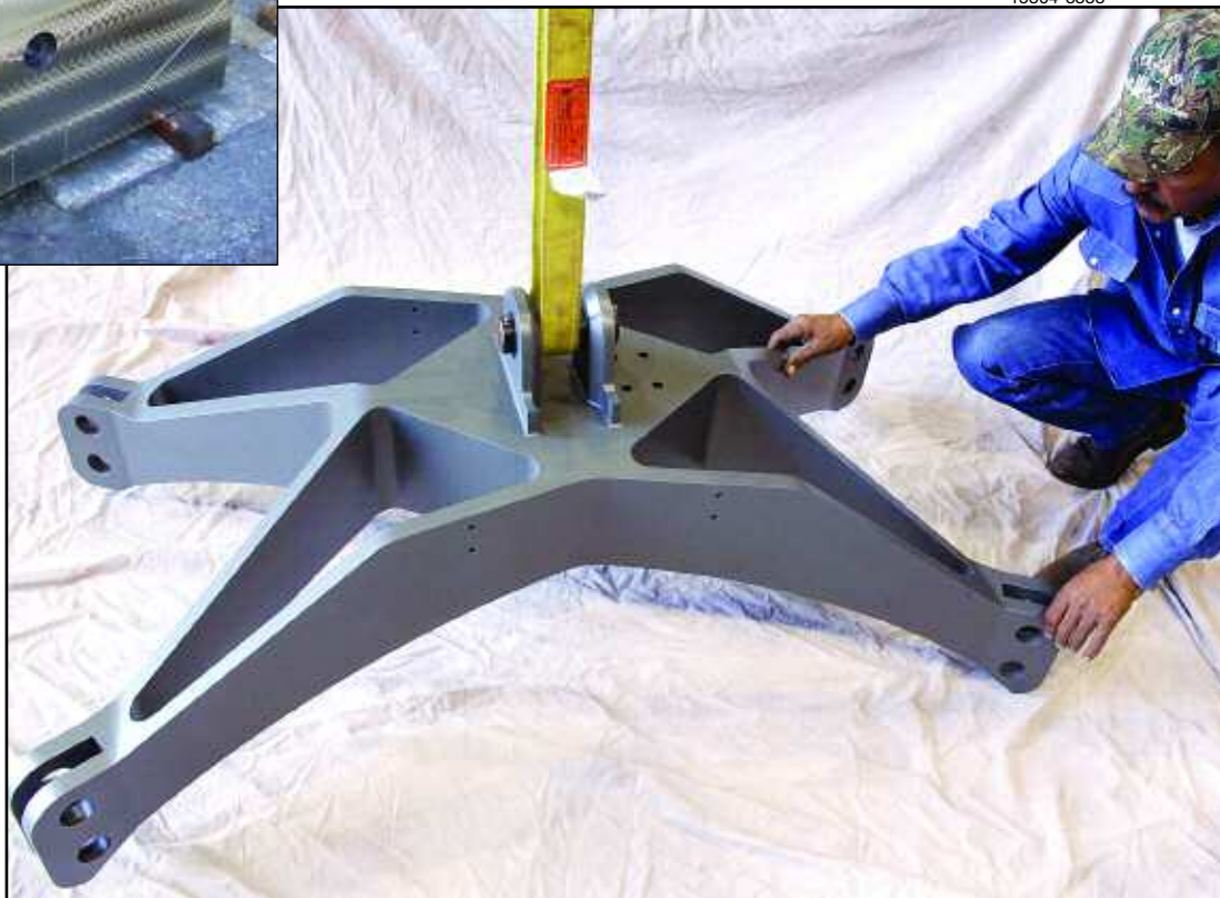
The lifting bridle was machined from a single large titanium 6Al-4V ELI alloy forging (top left). The bridle, which attaches to the rescue module hull, anchors the umbilical cable and also lifts the rescue module assembly.
