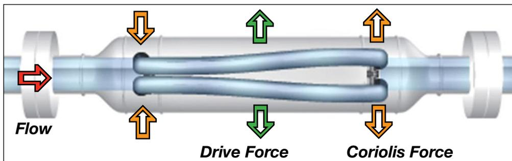
A top view of a dual-tube Coriolis meter shows an exaggerated twist in the flow tubes resulting from the Coriolis force generated by flow through the tubes in combination with the electromechanically driven tube vibration. When there is no flow, the tubes vibrate without being twisted.
