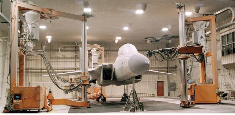
For more than 20 years, SwRI has been developing large robotic systems for aerospace coatings applications such as the robotic depaint system designed to maintain the U.S. Air Force's fleet of F-15 fighter jets. Current research has demonstrated that for some applications, a mobile solution can be less costly and more flexible.
