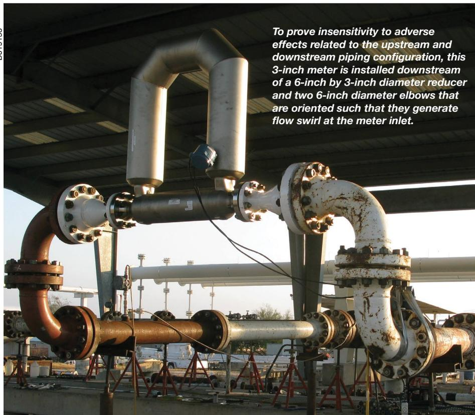
*To prove insensitivity to adverse effects related to the upstream and downstream piping configuration, this 3-inch meter is installed downstream of a 6-inch by 3-inch diameter reducer and two 6-inch diameter elbows that are oriented such that they generate flow swirl at the meter inlet.*
