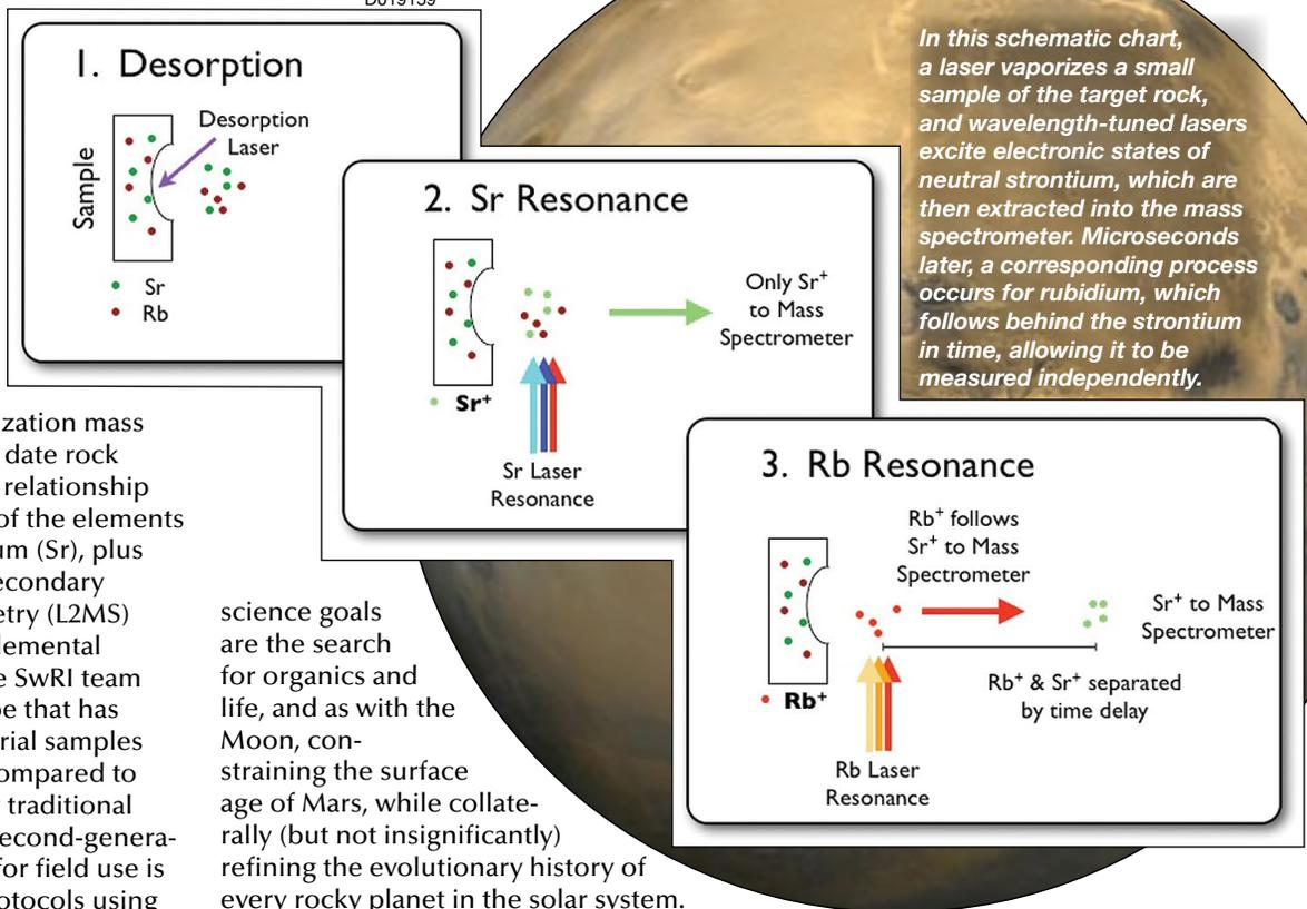
*In this schematic chart, a laser vaporizes a small sample of the target rock, and wavelength-tuned lasers excite electronic states of neutral strontium, which are then extracted into the mass spectrometer. Microseconds later, a corresponding process occurs for rubidium, which follows behind the strontium in time, allowing it to be measured independently.*
