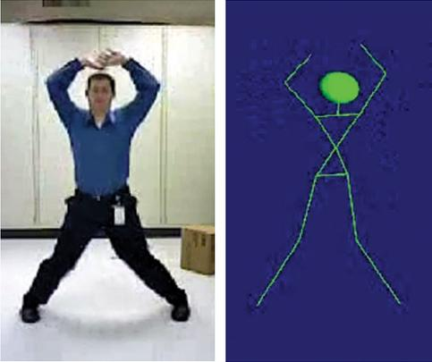
To recognize human actions, the SwRI-developed system tracks gross motions using skeleton models. A machine learning system, which has prior knowledge about different types of actions, can then classify the motion by type.
