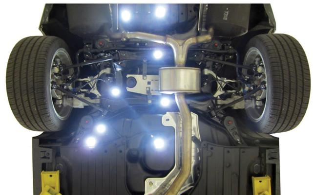
This research vehicle is equipped with SwRI's Ranger localization technology for automated vehicles. Using a ground-facing camera, illumination, and algorithms, Ranger allows for precise automated driving, accurate to within 2 centimeters.
