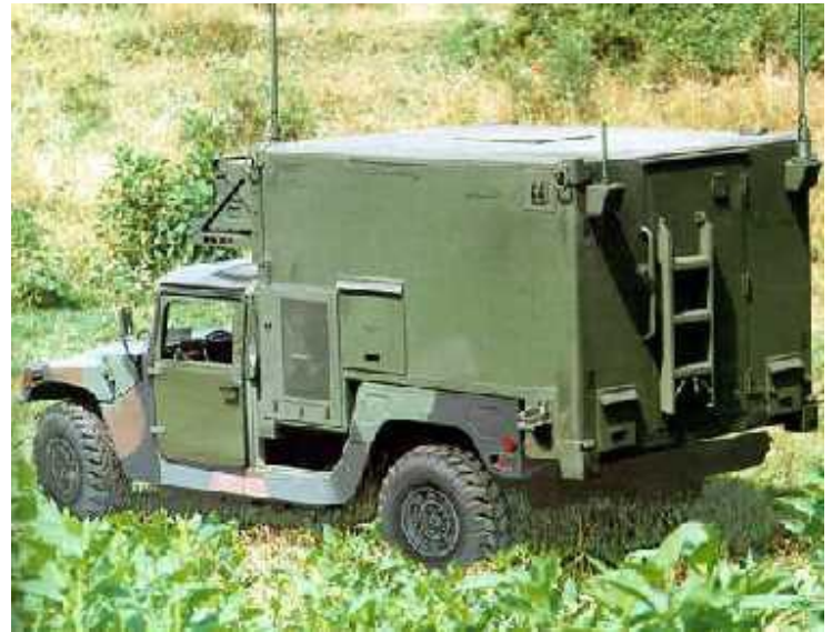
Petroleum Quality Analysis System Mobile Laboratory
