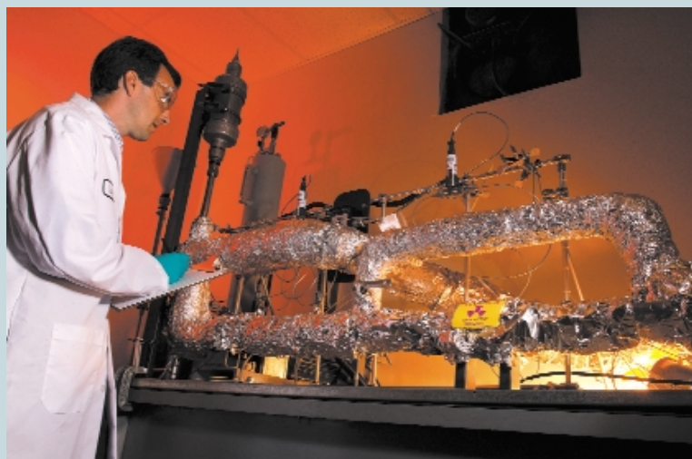
Real-time radioactive tracer flow loop simulating refinery conditions
