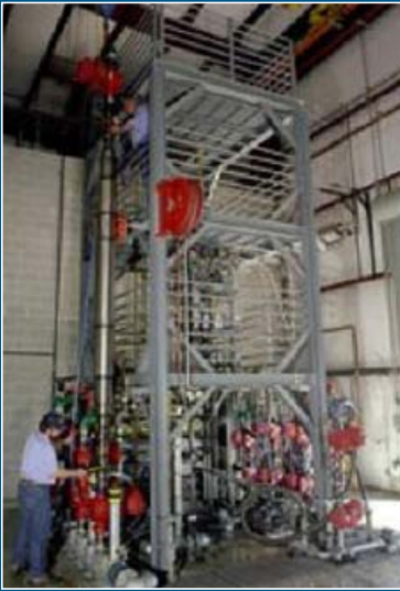
This test stand is used for liquid testing of safety valves and other flow products. Both water and sand slurry flows are available for use in testing.
