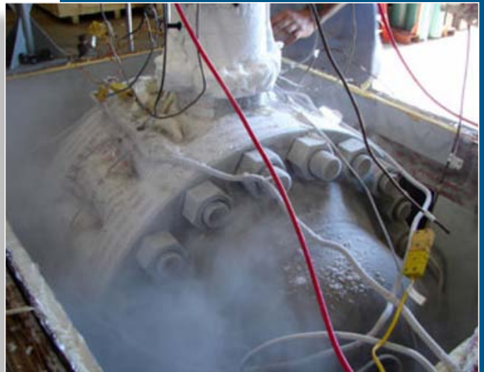
Testing is performed on a variety of products to determine operation and seal integrity at temperatures as low as -320^{\circ}\text{F} .
