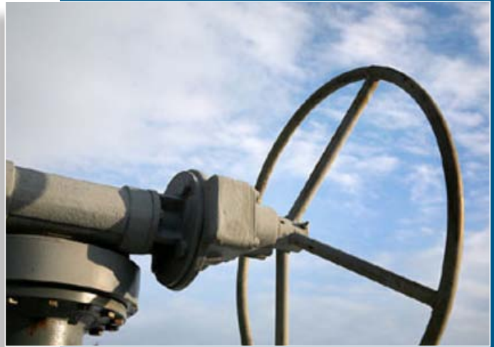
SwRI conducts fugitive emissions testing on valves and other products that handle greenhouse gases.
