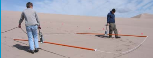
Geonics PROTEM 47 Transmitter and PROTEM 47D Receiver
