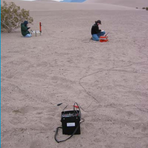
Geonics PROTEM 47 Transmitter and PROTEM 47D Receiver
