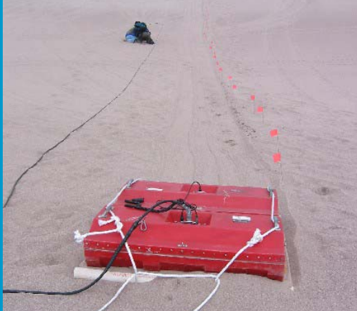
Multiple Low Frequency radar antenna (16–80 MHz)
