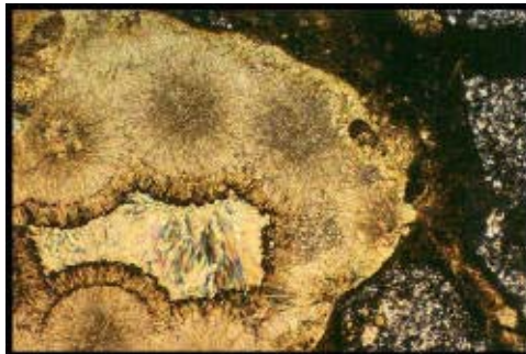
Transmitted light photomicrograph of radiating clusters of intergrown schoepite and uranophane. This is a replacement texture after colloform uraninite. Scale - 2.6 mm across
