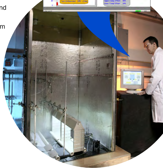
Variables such as temperature, humidity, corrosive salt solution, and ultraviolet radiation can be programmed dynamically to test requirements.
