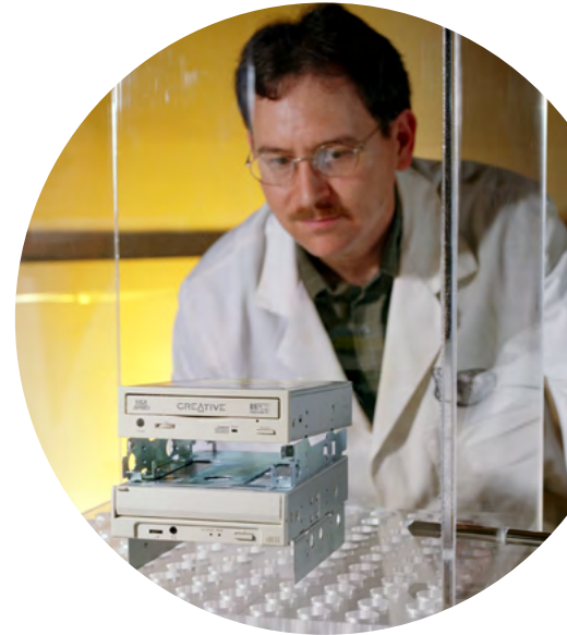
SwRI has developed a gaseous contaminants facility to test a wide range of materials and their ability to withstand exposure to atmospheric and industrial airborne pollutants on pollutants.
