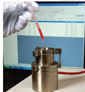
To determine fuel heat characteristics, SwRI staff conduct thermal conductivity tests.
