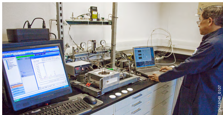
High-temperature CO 2 separation membrane evaluation system
