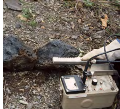
CNWRA scientists conducted field testing (left) to identify radiation hotspots for detailed sampling and characterization. Center scientists excavated a small abandoned slag pile (right) to collect fresh, unweathered samples for detailed laboratory analysis.
