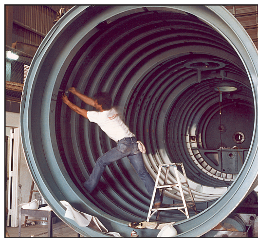
SwRI built the Kokanee submarine, the largest unmanned sub in the world (roughly 100 feet long and 10 feet in diameter), to simulate the acoustic and hydrodynamic characteristics of the Seawolf Class attack submarine. All of its structures, foundations, and control panels were designed and fabricated at SwRI.
