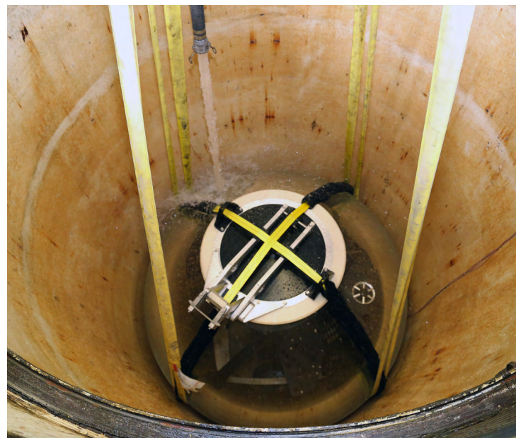
Pressure hull instrumented for external pressure test
