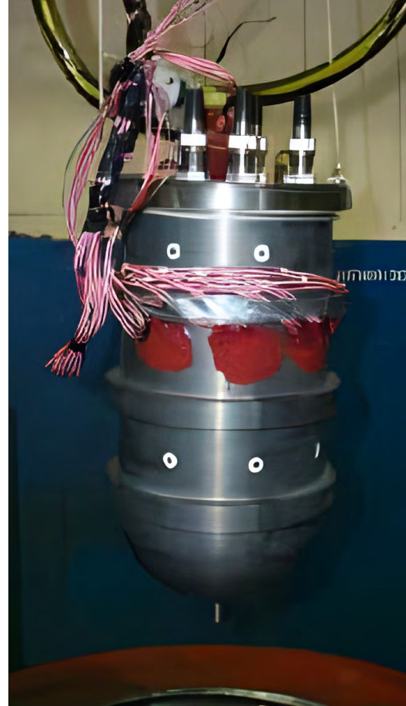
Instrument housing strain gaged prior to proof pressure test
