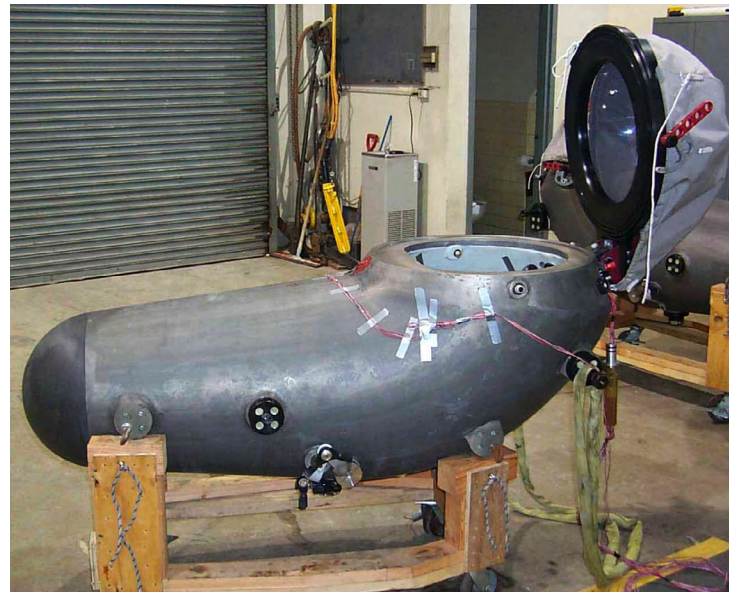
One-man submersible hull instrumented with strain gages for external pressure test to establish maximum depth capability
