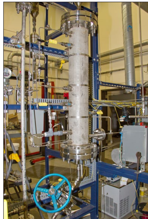
The reactor/riser is capable of processing diverse feed types such as solids, liquids, or highly viscous feeds.
