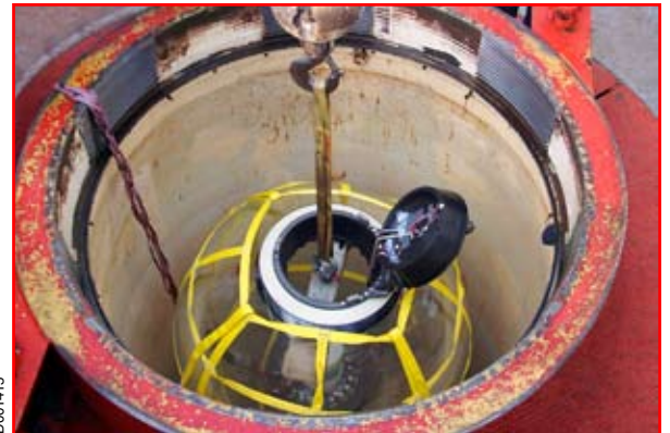
Acrylic pressure hull instrumented for external pressure test
