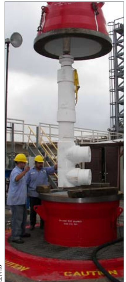
Subsea insulated pipe sample at 10,000-ft depth in 40°F salt water (internal pipe temperature 280°F)
