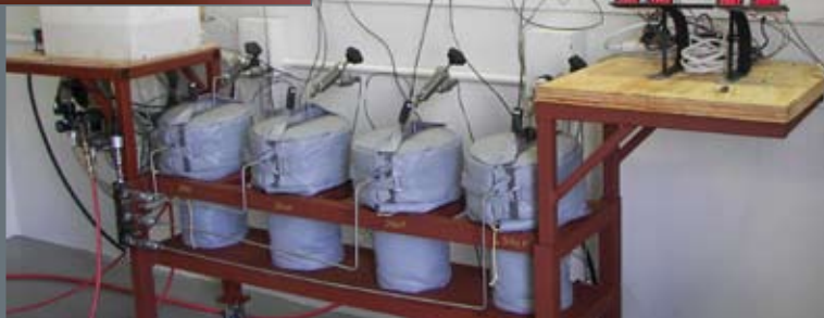
Hydroclave assembly for long-term exposure testing (Inset – Material test samples)
