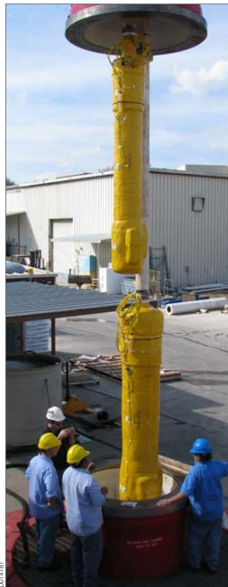
Simulated service insulation test samples being set up for pressure/temperature test
