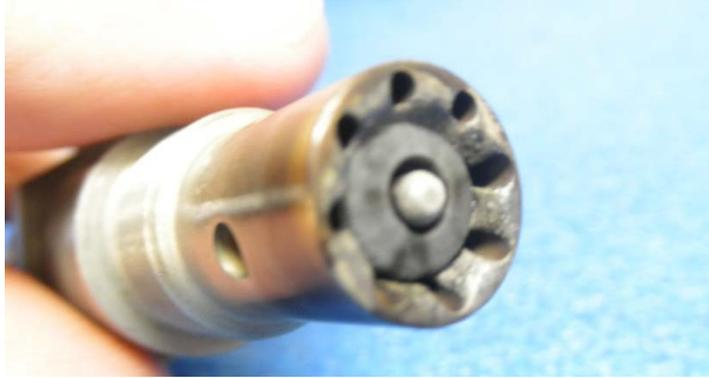
Figure 6. Dry Spark Tip, End of Test.
