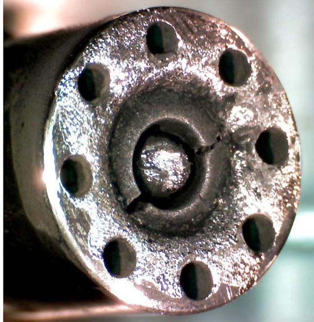
Figure 8. Wet Spark Tip, End of Test.
