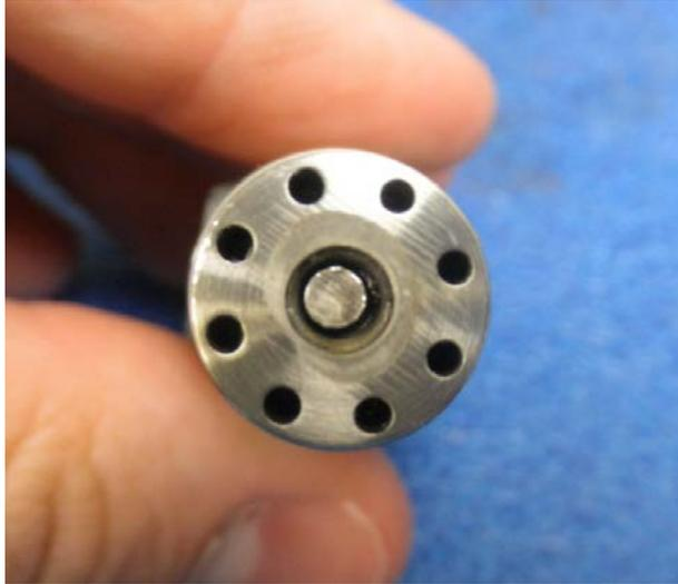
Figure 2. Igniter Tip with Ir Alloy Electrode.
