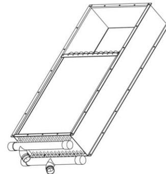
Figure 4. Cogen Heat Recovery Unit
