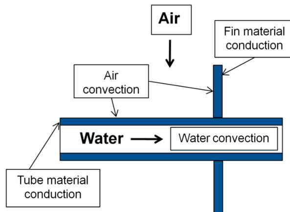
Figure 5. Heat Transfer Model
