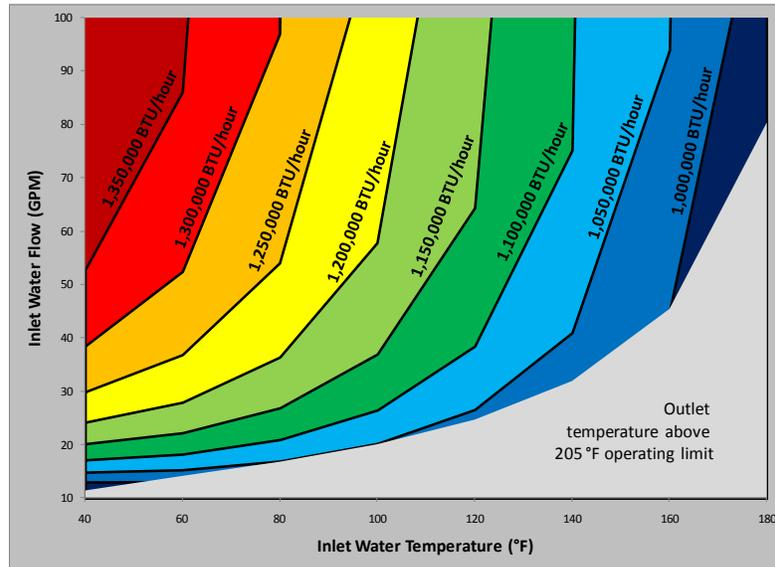
**Figure 6. Heat recovery unit performance curves**
