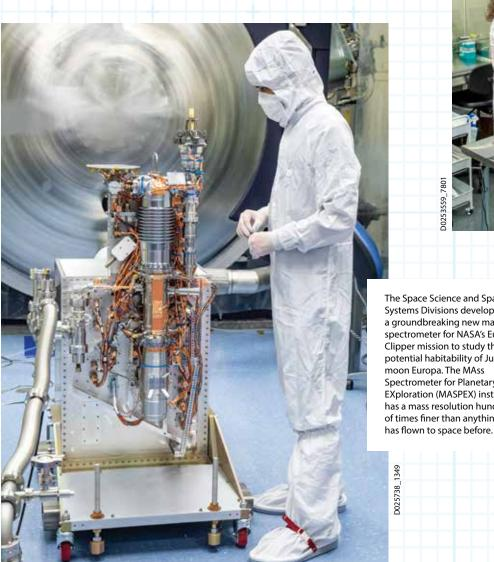
The Space Science and Space Systems Divisions developed a groundbreaking new mass spectrometer for NASA's Europa Clipper mission to study the potential habitability of Jupiter's moon Europa. The MAss Spectrometer for Planetary EXploration (MASPEX) instrument has a mass resolution hundreds of times finer than anything that
