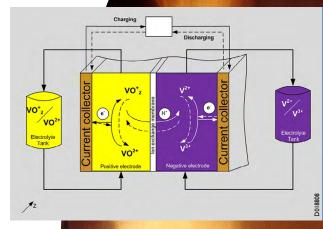
ESTC engineers have conducted research and development of electrolyte formulations, proton exchange membrane technology, mechanical fluid systems, and electronic control systems for a gridscale vanadium redox flow battery.
