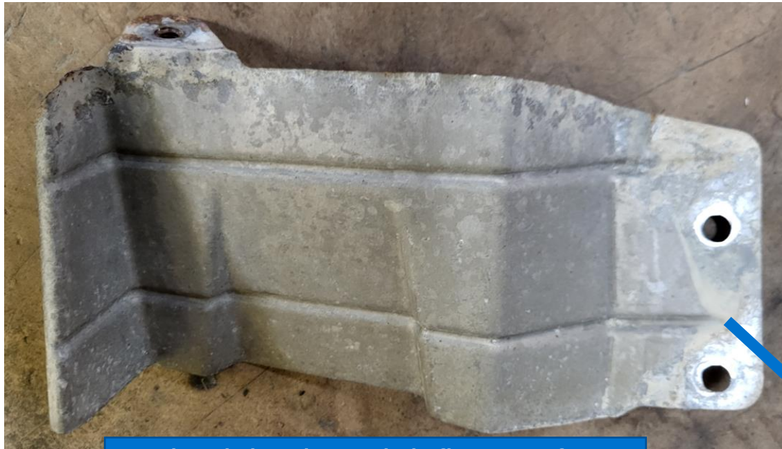
Aluminized steel deflector after vehicle level corrosion testing
