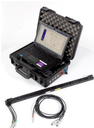
MsSRv5M instrument and -segment array on MsT 8x8 probe
