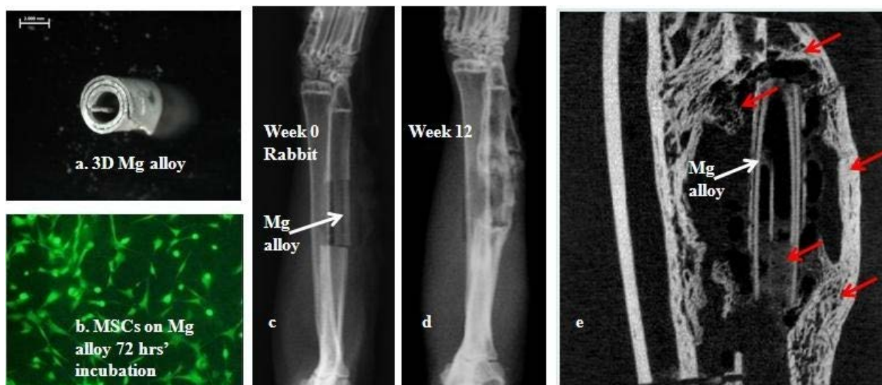
Figure 1. (a) 3D coated biocompatible Mg alloy scaffold (3.5 mm diameter x 15 mm length); (b) Image of live MSCs on coated Mg alloy; (c-d) Mg alloy scaffold implantation resulted in repair of a critical sized ulna
