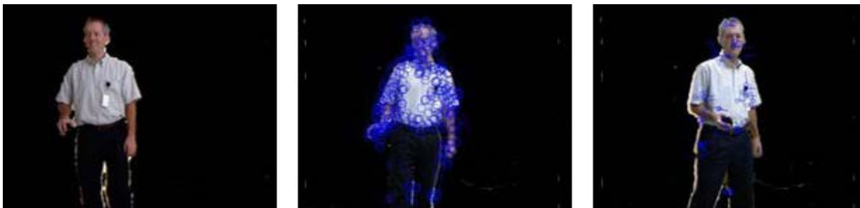
Figure 1. Colorized clouds of data from Microsoft's Kinect sensor are processed by a ROS node to first remove the background data (left). Then, a node detects and characterizes salient features (middle). Correspondence of features in subsequent frames helps estimate the subject's pose (right).
