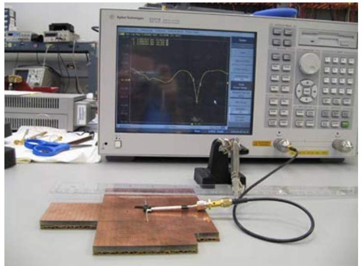
Figure 1. A dipole antenna in direct contact with a novel ground plane. The impressive return loss in this low profile system would be impossible using a conventional ground plane.
