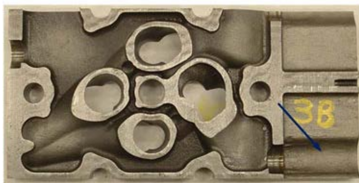
Figure 2. Post Fatigue Test Cylinder Head Section for Crack
