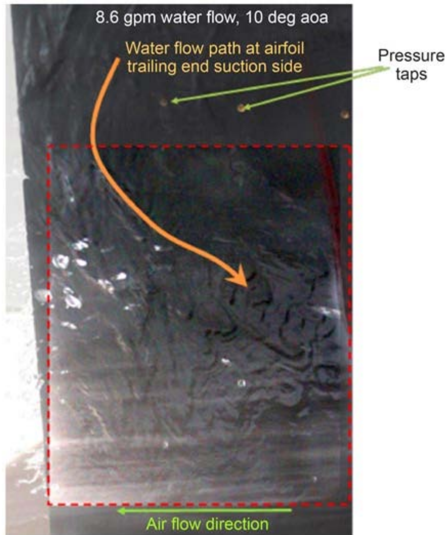
Figure 5. Baseline testing image shows liquid film interaction.
