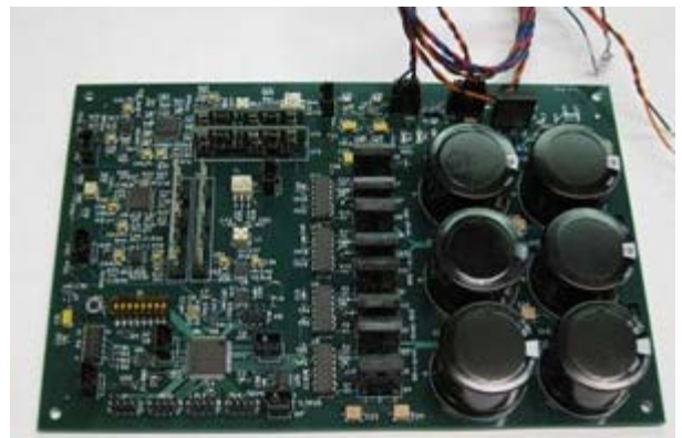
Figure 1. Dual channel pulser/receiver board final design, before installation in enclosure.
