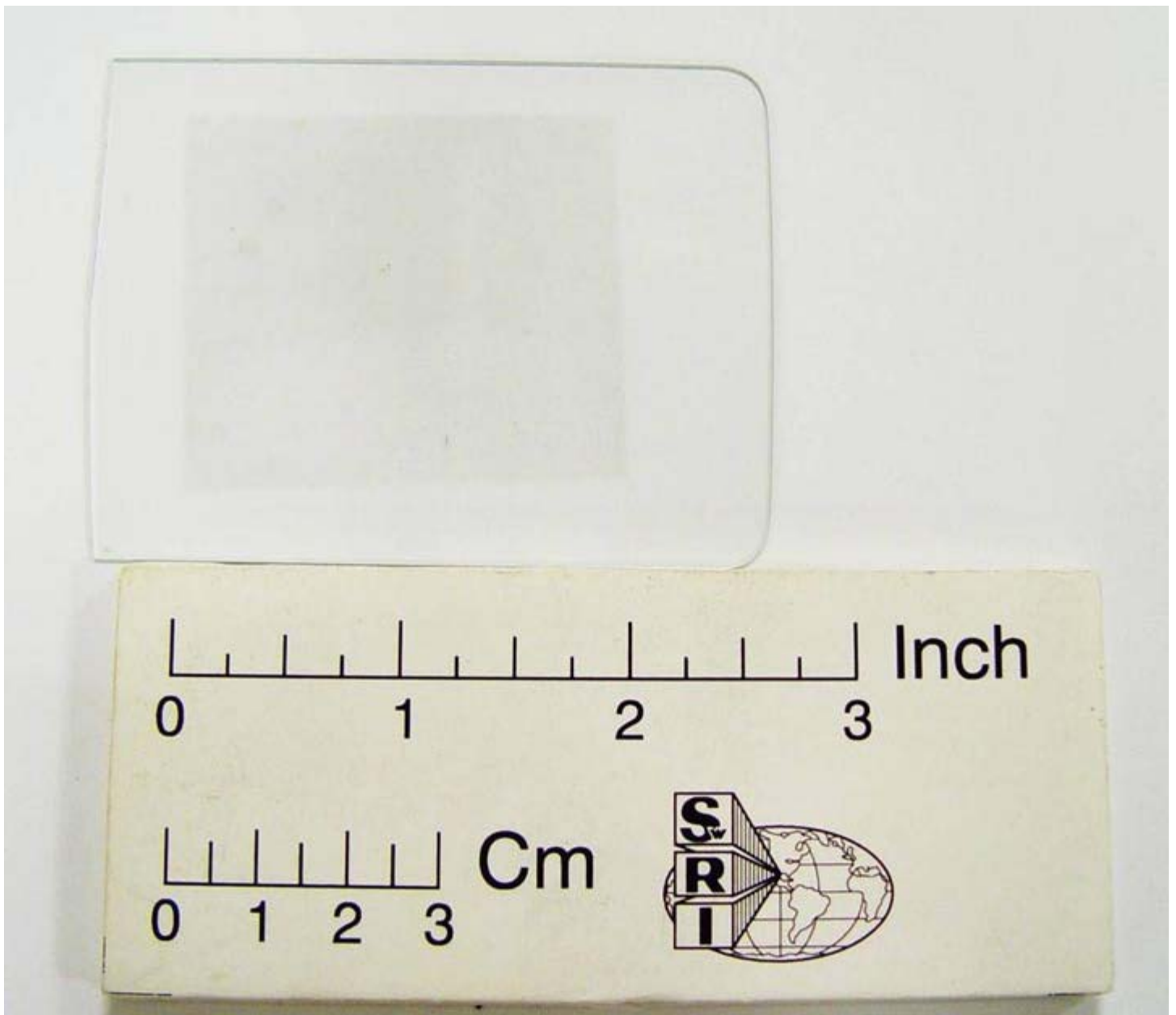
Figure 3. Photograph of 2 in. x 2 in. pristine graphene film transferred to glass substrate. Measured performance of 94 percent transmittance and 900 to 1,300 ohms/square for transferred SwRI graphene films.
