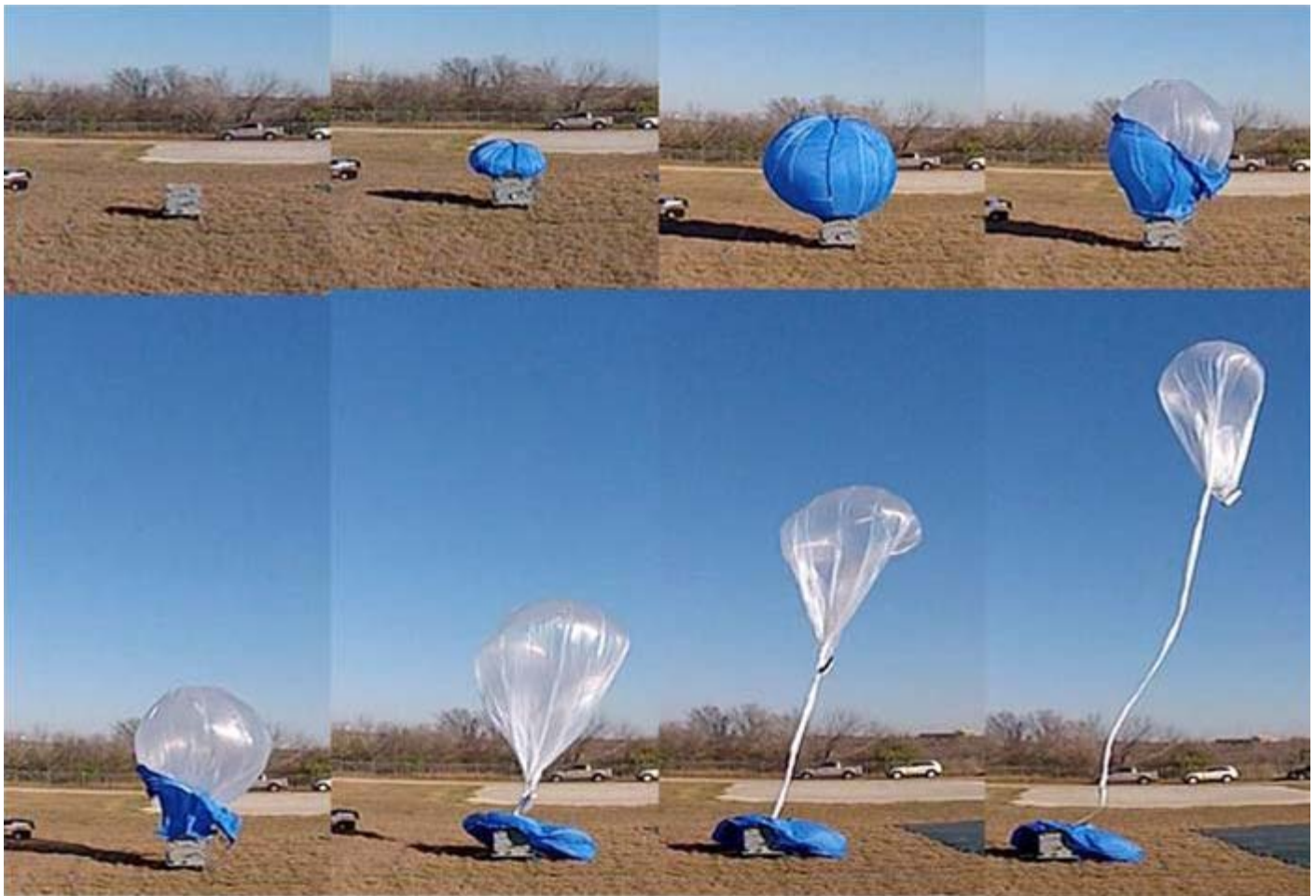
TALS Demonstration of an Automated Inflation and Launch of an Airship
