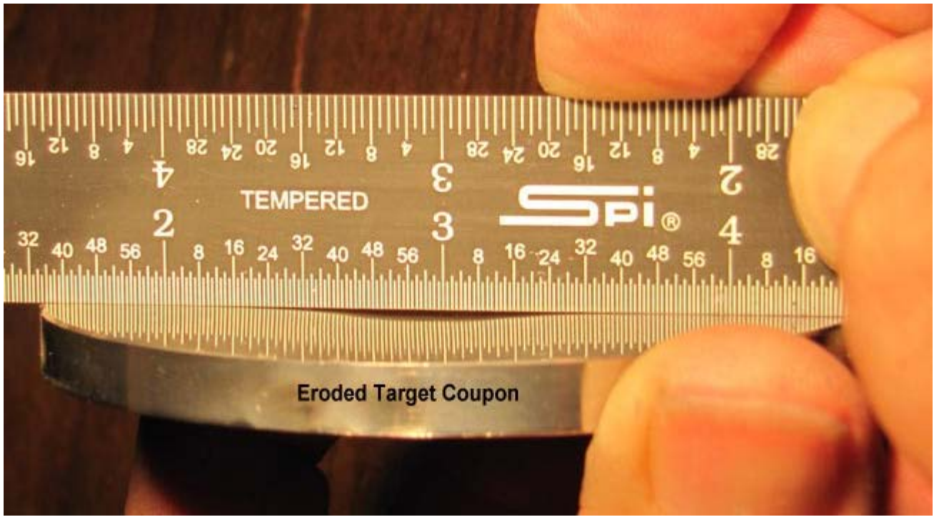
Figure 2. After running in the test rig for approximately 20 hours, the 316 stainless steel coupon shows clear evidence of an eroded indentation at the target face.
