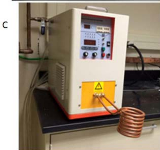
A. Particle size of a MCAp NP formulation. B. EDX analysis of a MCAp NP formulation that has high loading of iron oxide inside the CaP. *Note: Results do not include elements with Z < 11 (Na). C. Purchased bench top IHG061A induction machine (coils of different sizes are available). D. The induction heating capabilities of our prepared MCAp NP suspension in water (18.6 mg/mL). The MCAp NPs can be heated to 60°C within 6 min.
