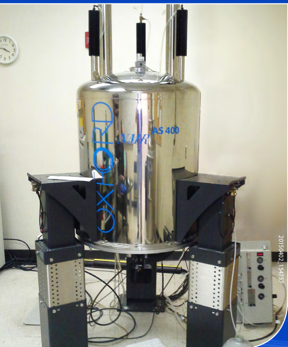
400 MHz Varian NMR spectrometer
