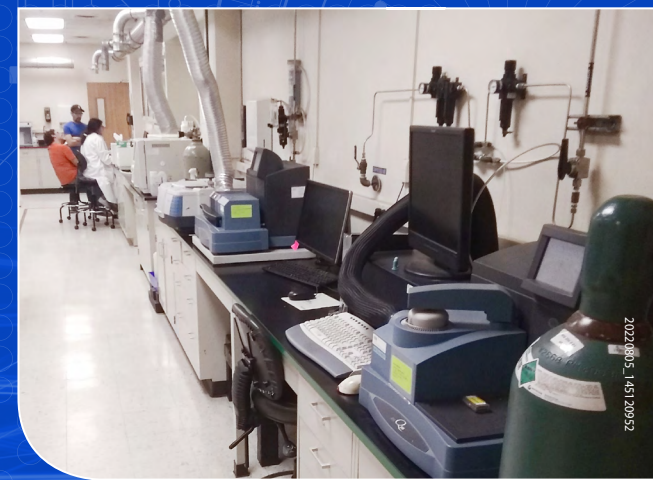
Thermal analysis: TA Instruments SDT Q600 and MDSC Q100; FTIR Nicolet iS50
