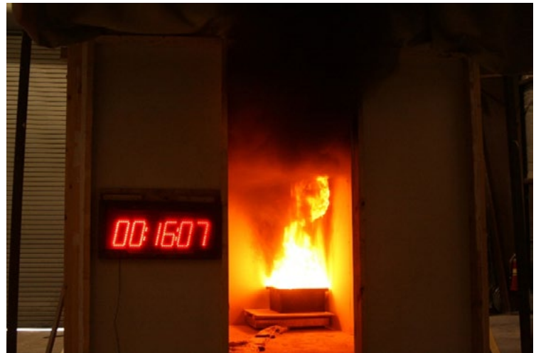
Liquid fuel pool fire test to quantify the effect of a wall or corner proximity on the burning rate
