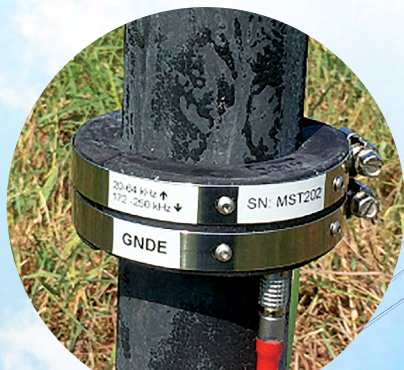
MsT probe for guided wave screening of buried rods.
