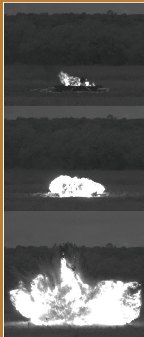
Catastrophic failure of a compressed hydrogen cylinder
