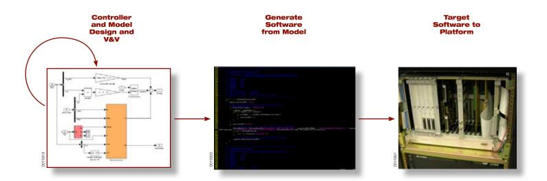
SwRI uses model-based design techniques as part of its system design process. Institute staff members create system models and controllers using the design tools and extensively test and evaluate their performance against the system requirements. In subsequent efforts, the design tools produce software which eliminates the need for manual conversion and reduces development time.
