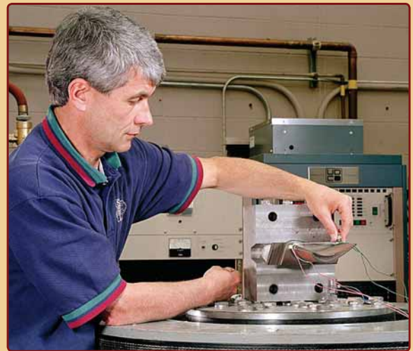
Instrumentation attached to a test item during vibration testing can aid in frequency response analysis.
