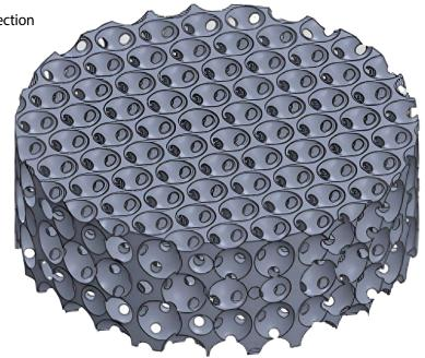
A novel, single-use 3D-printed bioreactor enhances surface-to-volume ratio and cell culture capacity.
