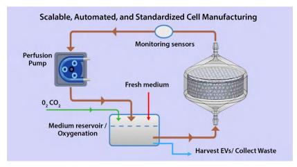
The structure supports automated, circulation-based cell culture driven by a pump, with a media reservoir utilized to maintain optimal levels of  $O_2$ ,  $CO_2$ , and nutrients.
