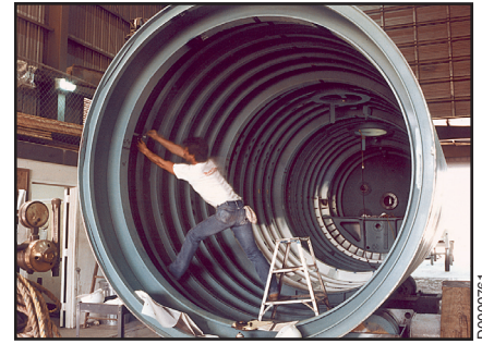
SwRI built the Kokanee submarine, the largest unmanned sub in the world (roughly 100 feet long and 10 feet in diameter), to simulate the acoustic and hydrodynamic characteristics of the Seawolf Class attack submarine. All structures, foundations, and control planes were designed and fabricated at SwRI.
