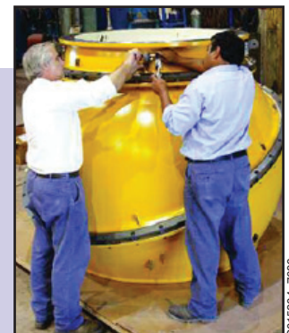
50-in ID, 24-ft long, 6,500-psi deep ocean test chamber at SwRI
